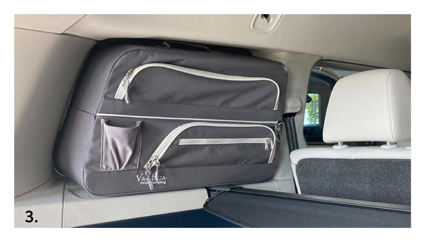
First press the packing bag into the window at the top, then at the bottom, so that the bags are firmly positioned on the bottom of the trim panel (pic. 2 + 3).
